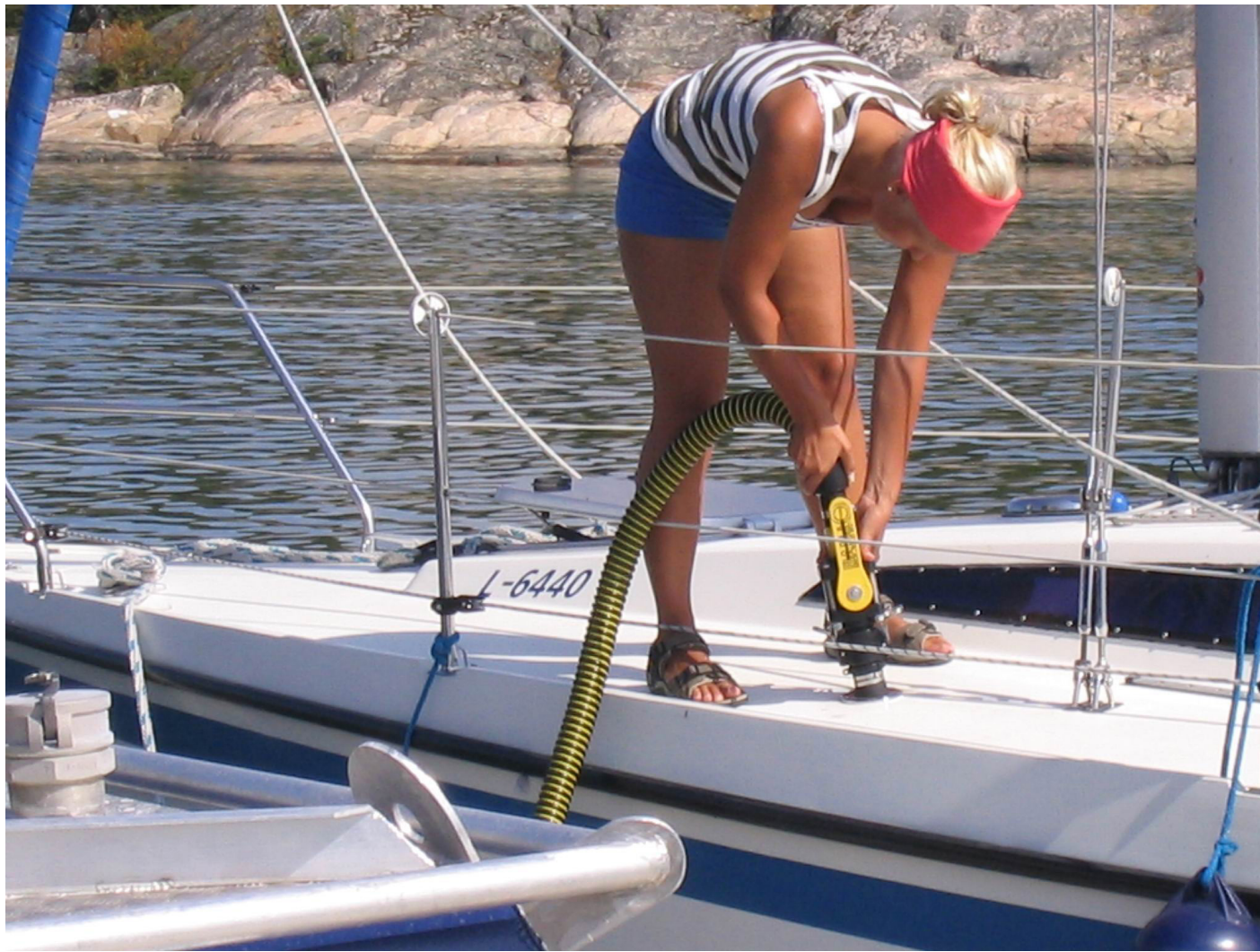
Fig. 14: Emptying the boat's septic tank. / Keep the Archipelago Tidy Association
