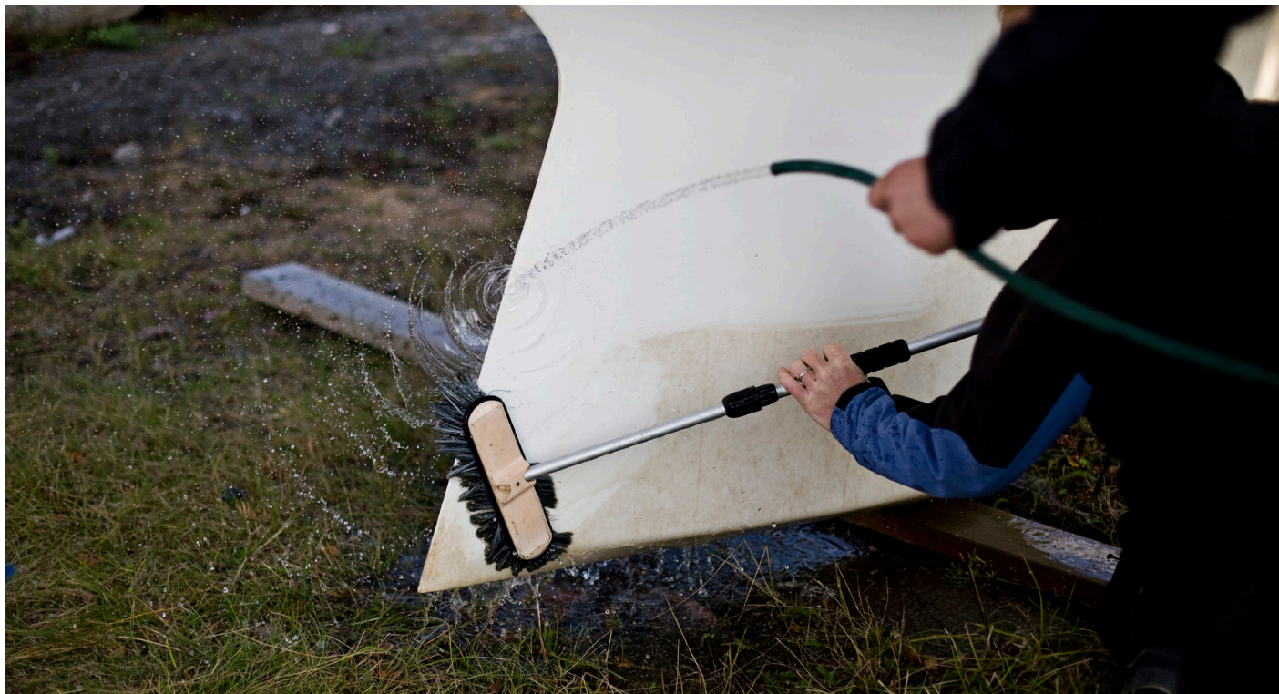
Fig. 12: Boat cleaning with a brush and a water hose. / Keep the Archipelago Tidy Association
