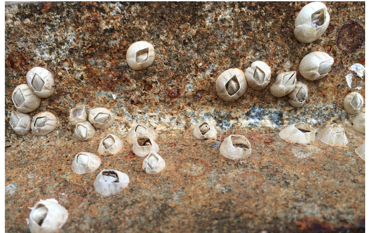
Fig. 11: It is recommended to brush or scrape off the barnacles from the boat hull. / Keep the Archipelago Tidy Association
